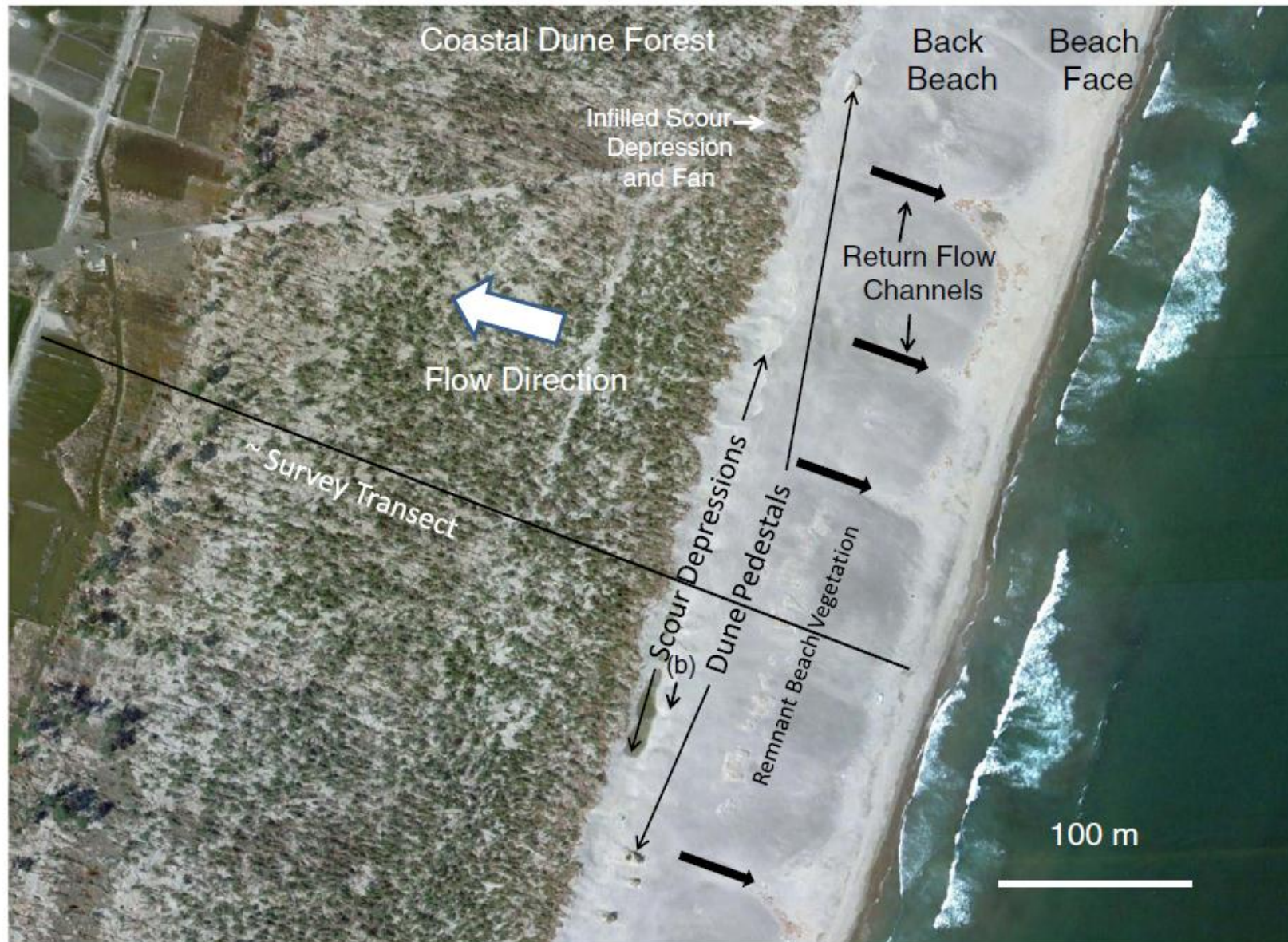
Fig. 5. Google Earth image taken 4/5/2011 showing the survey transect line, remnant artificial dune pedestals and associated shore-parallel scour depressions, probable si partially-infilled return-flow channels on the beach face and average flow direction as determined from bent pine trees.
